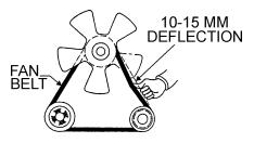
Figure 37. Fan Belt Tension
